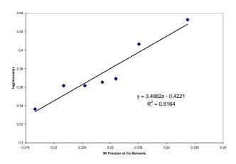
Figure 2. Logarithm of viscosity vs. weight fraction of co-solvent.
