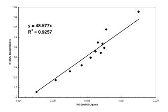
Figure 1. Logarithm of transmittance vs. dye concentration.
