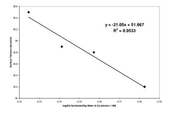
Figure 3. Surface tension vs. logarithm of surfactant concentration.
